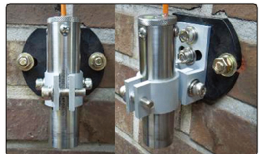
[Installation of foil strain gage inclinometer]
