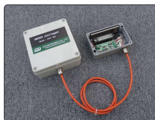
[ELS inclinometer connection]
