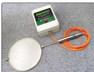
[Measurement of earth pressure]
