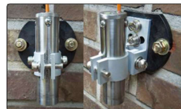
[Installation of VW inclinometer]
