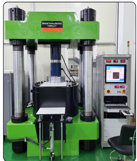
[1200ton-f Material testing machine]
